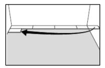
4. Fold the panel down, pressing lightly on the left. Check that the board is well joined to the top one.
