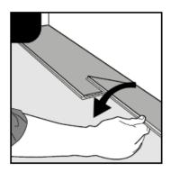
**2.** To engage the locking system, press the end of the board until you hear a click. A click indicates that the locking system is properly engaged.
