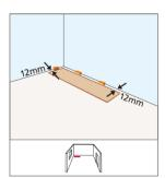
Floating floors require freedom to expand and contract without binding or rubbing on vertical surfaces. It is very important that there be enough expansion gaps between the flooring and all the walls.
